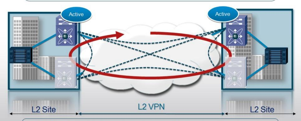
A solution that natively provides automatic detection of multi-homing without the need of extending the STP domains is key.
