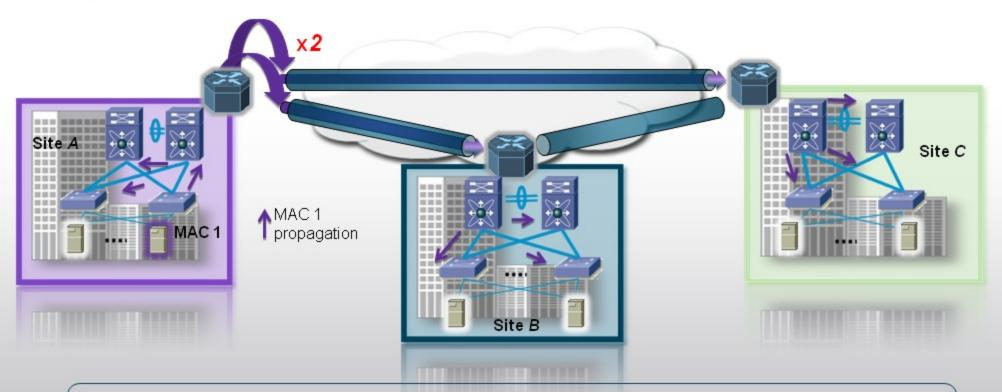
A solution that provides layer 2 connectivity, yet restricts the reach of the flood domain is necessary in order to contain failures and preserve the resiliency.
