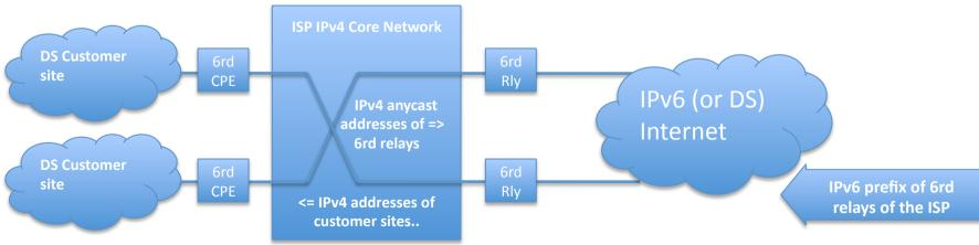
CPEs learn configurations (prefix, relay address etc) by manual configuration or via DHCP.
