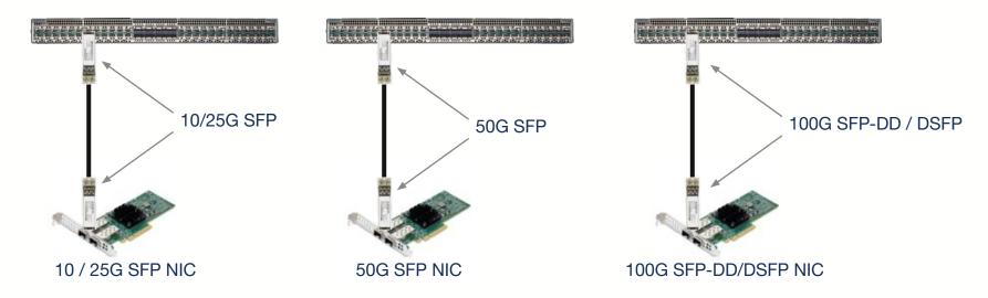
Note: a 100G SFP-DD / DSFP cannot be used in a 10G/25G/50G SFP port
